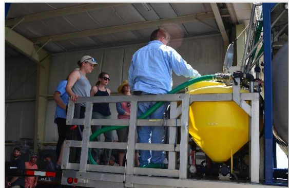
Demonstrating rapid loading and rinsing 2.5-gallon herbicide containers for helicopter applications.
