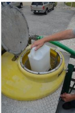
Demonstrating rapid loading and rinsing 2.5-gallon herbicide containers for helicopter applications.
