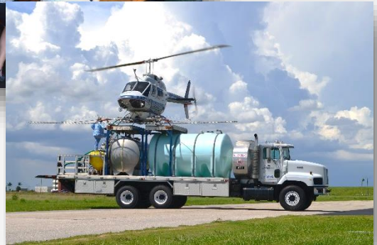
Left to right: Explanation of the various nozzle aper-tures designed to control droplet size and placement. Support vehicle with self-contained herbicide concen-trate and diluent tanks and landing/loading platform.
