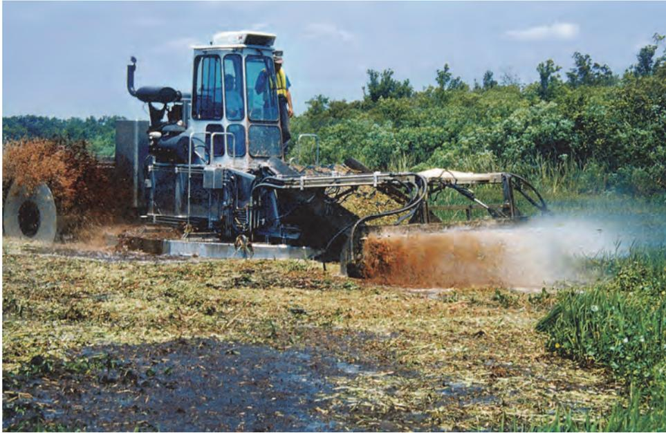
have been tested for chopping and shredding floating and emergent plants. Similar to other mechanical control equipment, shredder boats are very specialized pieces of equipment, are non-selective and create many plant fragments. However, they work well when used in the areas for which they are designed and are frequently used in wetland restoration projects, where removal of cut vegetation is too expensive or not feasible.
